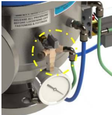
Figure 11 Tap turned to to outlet pressure
