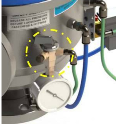
Figure 10 Tap turned for inlet pressure
