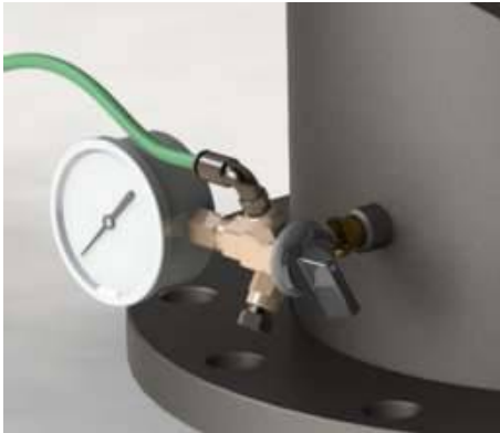
Figure 10 - Tap turned for inlet pressure.
