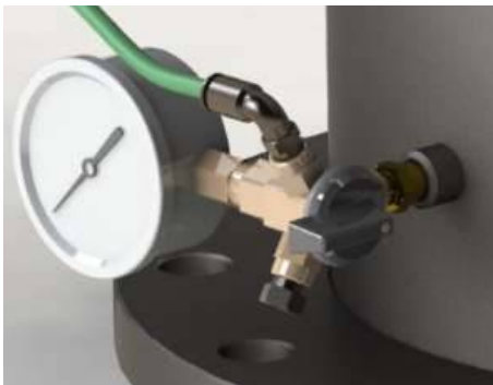
Figure 11 - Tap turned to outlet pressure.
